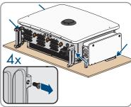
6. If the inverter is to be hooked into the mounting bracket using lifting gear, screw the eye bolts into the 2 upper threaded holes on the right-hand and left-hand side of the inverter and attach the lifting gear to them. The lifting gear must be suitable to take the weight of the inverter.
