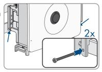
11. If the inverter was hooked into the mounting bracket without lifting gear, remove the carrying handles from the threaded holes on the right and left side.
