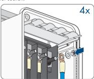
12. Place the grounding conductor incl. 1 washer and hex nut onto the stud bolt (M8, torque: 20 Nm to 30 Nm) in the middle section. Now tighten it all using a ratchet.
