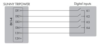
Figure 9: Connection of a remote terminal unit to the digital input DI D1-D4, Vcc of the Sunny Tripower.
