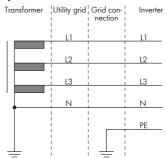
Figure 5: Overview of approved grid configurations
