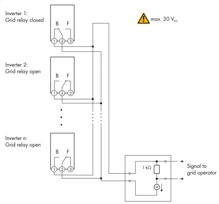
Figure 13: Wiring diagram for signaling the switching status of the grid relay (example)
