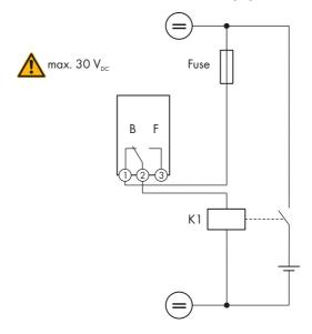
Figure 12: Wiring diagram for connection for controlling a load or for the power-dependent charging of the batteries
