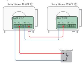
Figure 10: Example of the circuitry for connecting a trigger contact for the fast-stop function and linking multiple inverters
