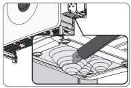
8. Route the cable through the sealing plate for the AC connection into the device.
